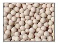
Each air dryer tank is filled with desiccant tablets, a chemical drying agent for deliquescent dryers. These dissolvable tablets are the most effective way to remove moisture from compressed air.
