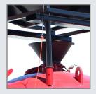
The steep angle of the 90° cone bottom provides significantly improved abrasive flow versus a 60° cone bottom.
