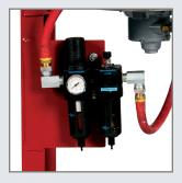
Pneumatic models include an easily accessible pressure regulator, particulate and moisture filter, and lubricator, which can be adjusted to regulate the volume of air and oil supplied to the fan for optimal performance.
